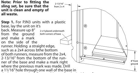
the location marked. Repeat this step for the inside surface of the runner (see diagram to the left). Repeat this procedure for the outside and inside surfaces of the other runner. When all 4 holes have been drilled,
